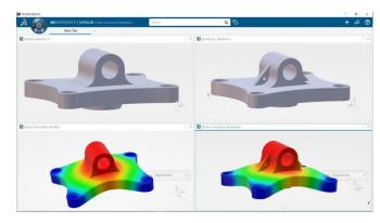
Easily compare the results of linear structural simulation during the design process.
