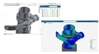
Transfer geometry and model features from SOLIDWORKS to Structural Performance Engineer with a single click to perform advanced simulation studies.
